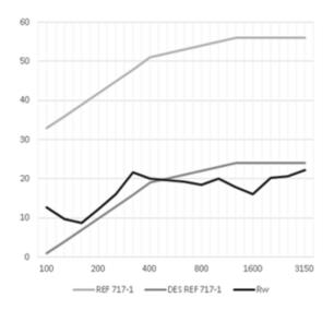
This graph shows the values of the sound reduction index R for the frequencies 100, 125, 160, 200, 250, 250, 315, 400, 500, 630, 800, 1000, 1250, 1600, 2000, 2500 and 3150 Hz.
