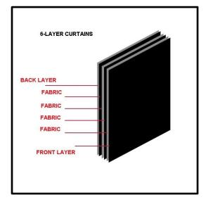
Our 6-layer curtains consist of a visual top layer, four middle layers and a back layer.
