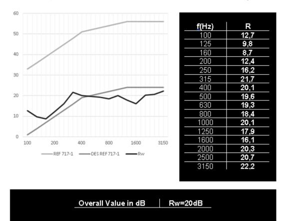
Both the graph on the left and the tables provide information on the sound insulation level of the curtain.
