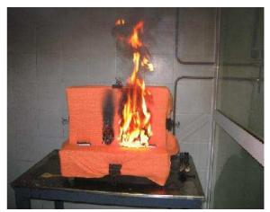
BS 5852 "Methods of test for assessment of the ignitability of upholstered seating by smouldering and flaming ignition sources: cigarette / flame / cribs". – Included at British Furniture & Furnishings (Fire) Safety Regulations, as well as on the hazard risk assessment specific standard BS 7176.
